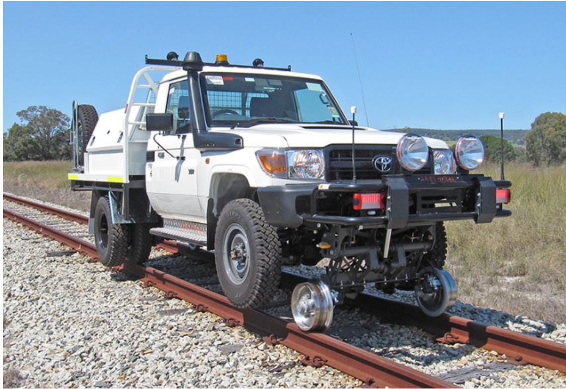
Figure 2. A Hi-Rail vehicle on tracks. The front rail wheels go behind the front bumper when retracted.
